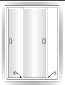
Adjust the operating panel with the screw at each end.
